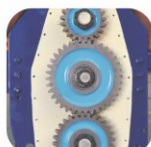
Side Geared Transmission: Positive drive -No shock load on tractor
