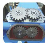
Multi-speed gearbox-4 speed options
